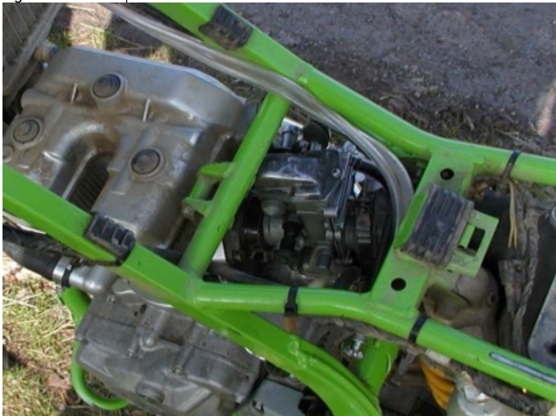
Figure 17: The completed carb install with breathers re-routed.
